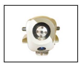
2) Slide the cowl in position on the fuselage. Use M3x10mm screws to secure the cowling to the fuselage.
