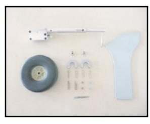
2) Install Retractable landing gear at the wings.
