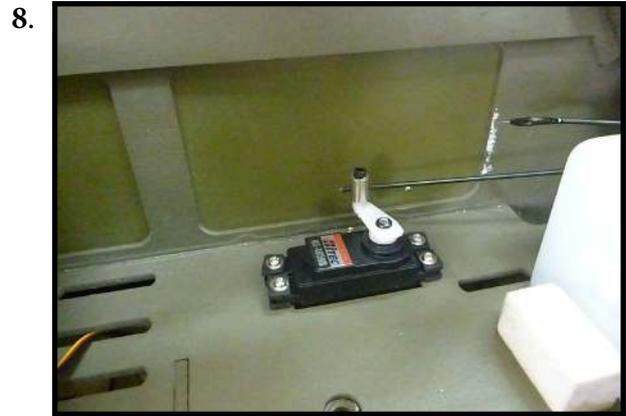
Move the throttle stick to the closed position and move the carburetor to closed. Use a 2.5mm hex wrench to tighten the screw that secures the throttle pushrod wire. Make sure to use threadlock on the screw so it does not vibrate loose.
