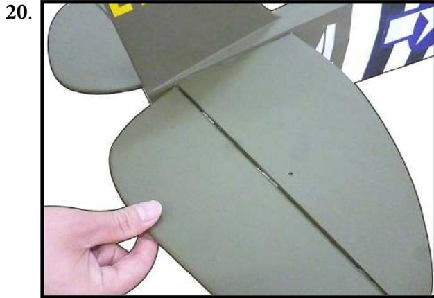
Check the alignment of the elevators in relationship to the stabilizer at the tips. There should be enough gap between the balance tab and stabilizer to they can move freely.
