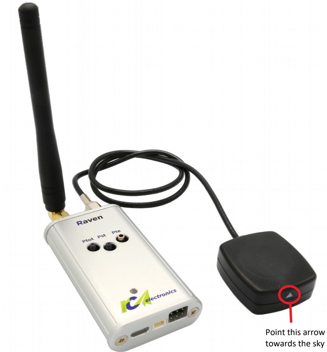
Figure 4: Correct position of GPS antenna
