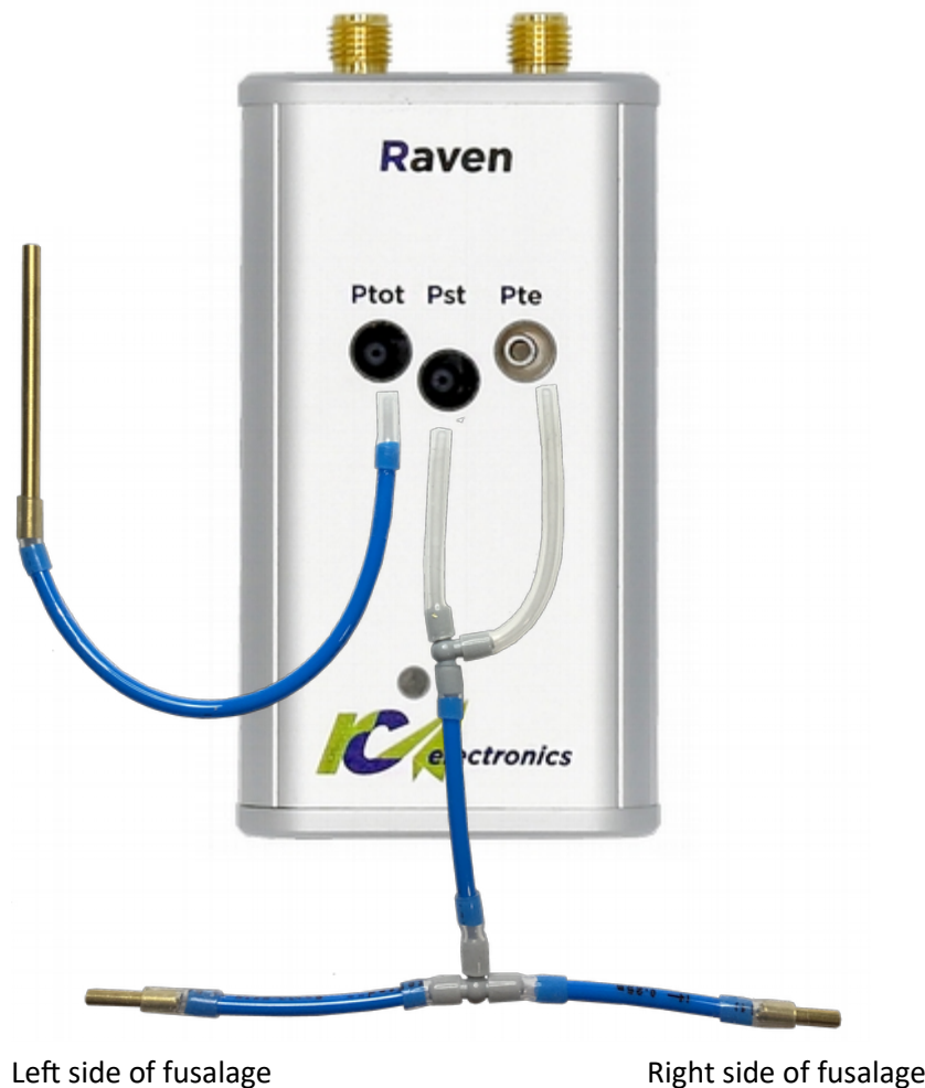
Figure 5: Example how to connect tubing with electronic vario compensation
