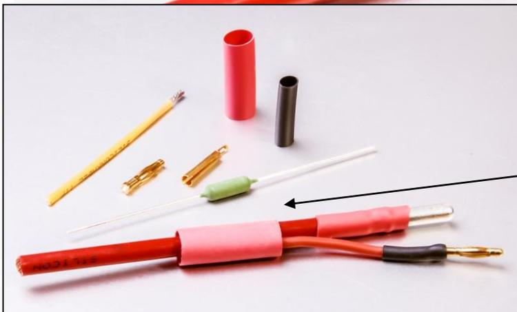
Isolate the resistor with the red shrinking tube.
