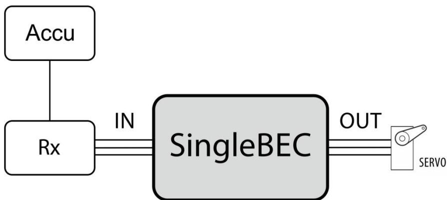
Fig. 1: Application wiring of SingleBEC
