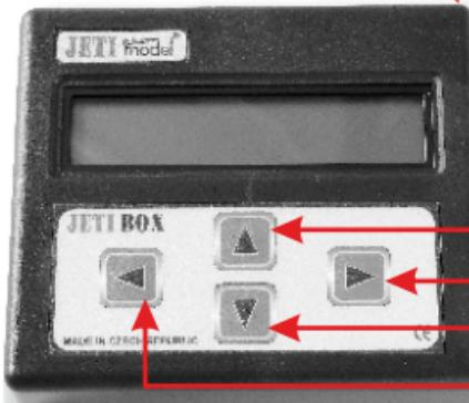
**Button UP U****Button RIGHT R****Button DOWN D****Button LEFT L****JETIBOX**
