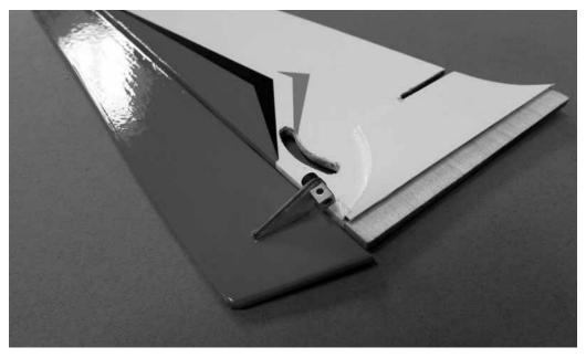
The screw-lock connector in the rudder horn illustrated in the instruction manual is mounted to the wrong side of the horn. Mount the screw-lock connector to the **bottom** of the horn as illustrated in this photo.
