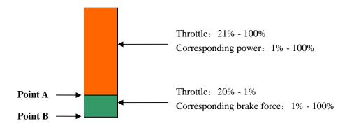
1) Simple settings: By setting the value in the bottom of the End Point of Throttle Channel can reduce the brake force. For example, set the End Point to be 90%, corresponding brake force will be 50%. (Prerequisite: Throttle range of ESC and throttle range of Transmitter should have been matched. Details refer to ESC Manual.)
