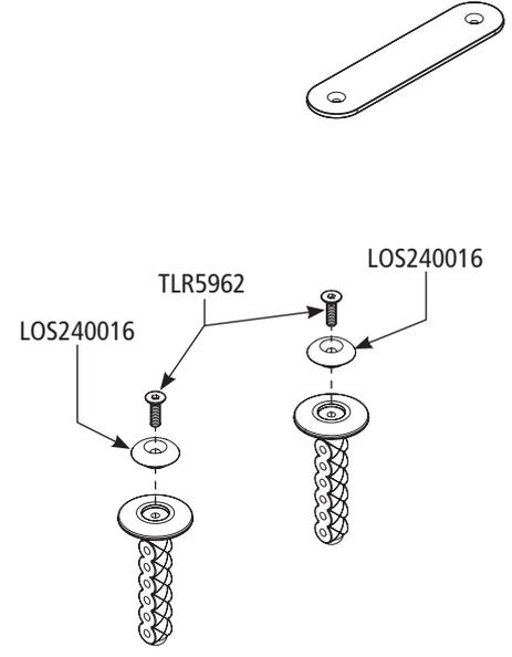
**Body Mounting Option 3:** Hard mounted body. Body is secured to the body mounts with screws and body buttons.
