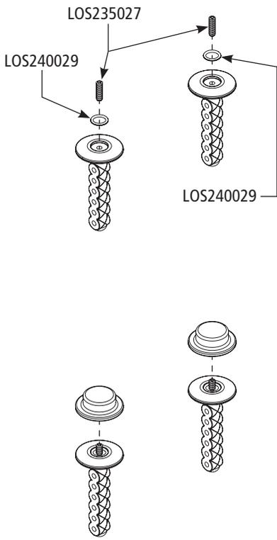
**Body Mounting Option 1:** Screw on style body mount uses a screw top to secure body to body mount post.
