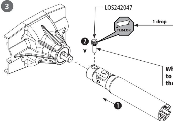
When installing the center drive shaft, be sure to align the screw side of the screw pin with the flat on the out put of the pinion gear.
