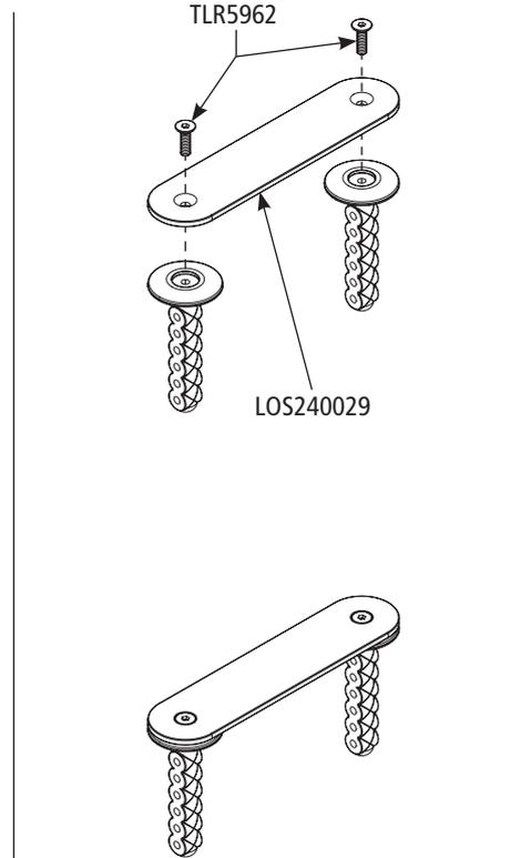
**Body Mounting Option 2:** Hook and Loop body mount. Use the cross bar mounted to the body mounts to apply hook and loop so you can mount your body without drilling any holes.
