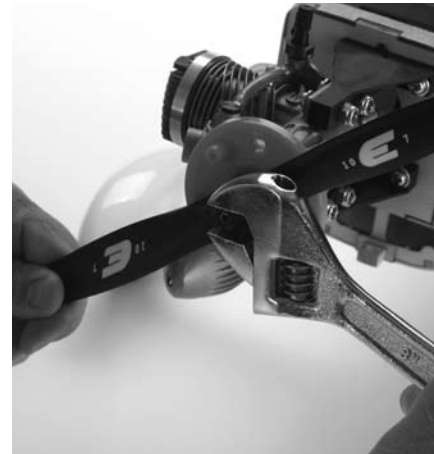
Securely tighten the prop nut using an adjustable wrench.
