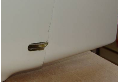
Rudder horn with M2 clevis
