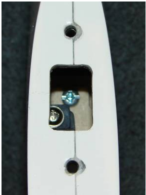
Screw the servo holder with two wood screws
