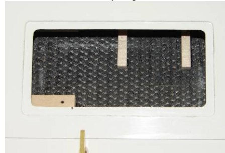
Glue with 5-min Epoxy
