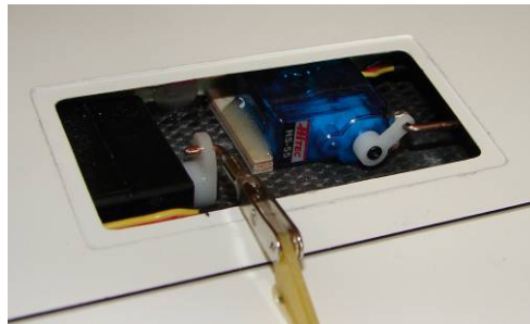
Glue the servo with 5-min Epoxy
